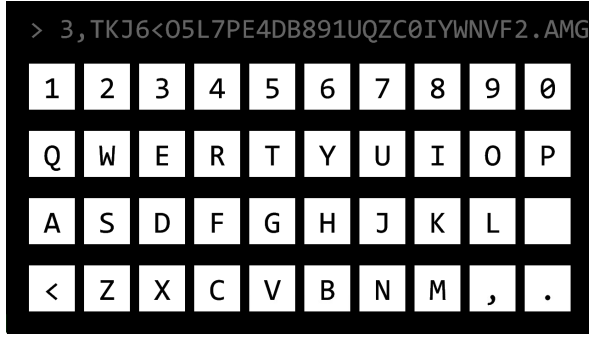
Fig. 2. Virtual keyboard for the 40-target SSVEP-BCI speller used in both the offline and online experiments. (A) Layout of a character input speller with 10 digits, 26 letters of the English alphabet, and four non-alphanumeric signs. The topmost rectangle is designed to show online feedback. (B) The tagged frequency and initial phase corresponding to each target are encoded by the joint frequency and phase modulation, respectively.
